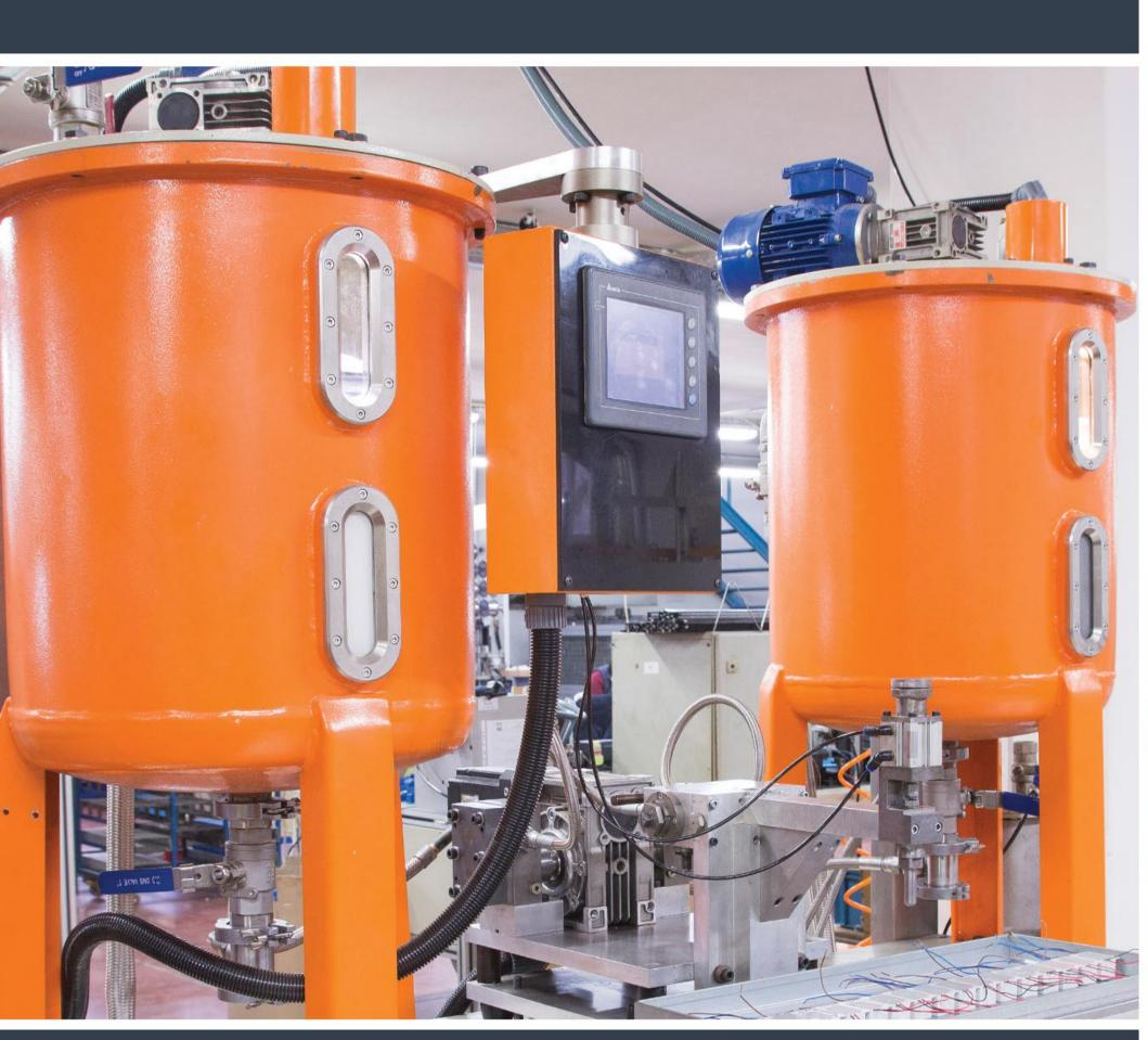
When there is a need for high-capacity production, extra preparation tanks need to be integrated into the system so that there is no waiting time for material preparation between shifts. After the ready material stock is finished, the homogeneous degassed material, is transferred to the casting tanks with the temperature-controlled feeding line and uninterrupted production is obtained.
